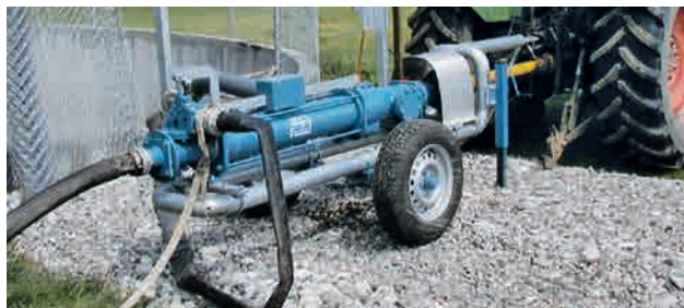
Umbilical system from a liquid manure tank with a pump from the WANGEN GL-series
