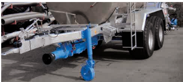
PTO pump on liquid manure tank / pump tank wagon
