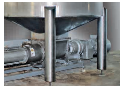
Feed process in a KL100RL120-8 V4A progressing cavity pump
