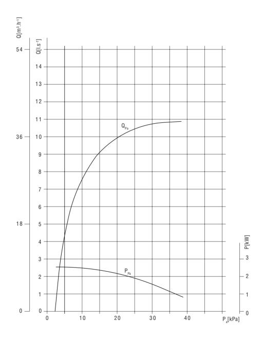
The performance curves are valid for clean air of temperature T = 20 °C, temperature of working (cooling) water T = 15 °C and at barometric pressure 101.3 kPa.
