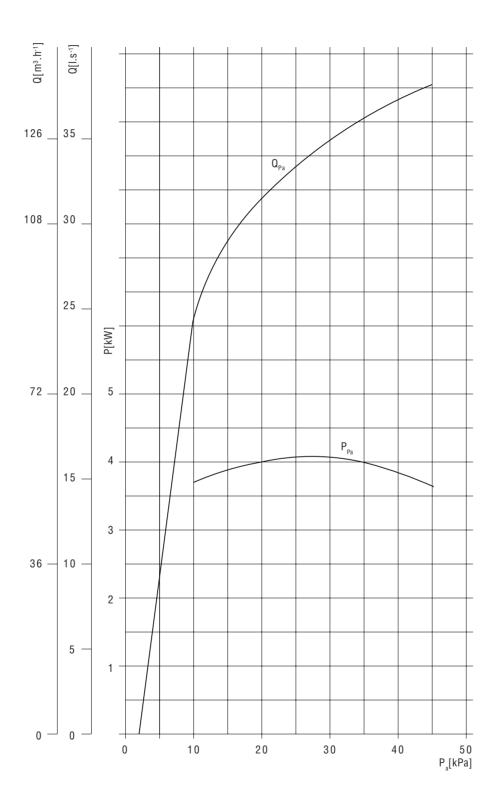
The performance curves are valid for clean  $\,$  air of temperature  $\,$  T = 20  $\,$  °C, temperature of working (cooling) water T = 15  $\,$  °C and at barometric pressure 101.3 kPa
