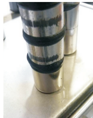
Finest debris collected on magnetic filter rod
