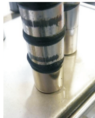
Finest debris collected on magnetic filter rod
