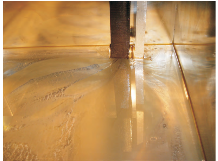
The floating oil will be attracted towards the oil skimmer
